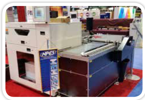
Bourg Sheet Feeder BSF working In-Line with a Rollem JetSlit card sliter
