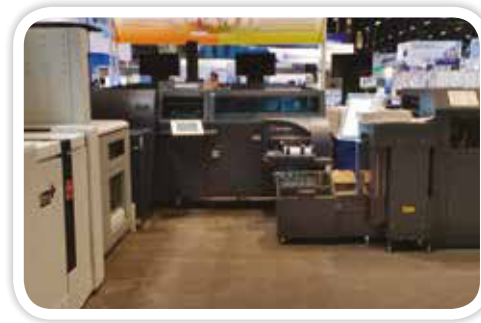
Océ VarioPrint 6xxx series working In-Line with a Bourg Binder BB3202 and a Three-Knife Trimmer CMT-130
